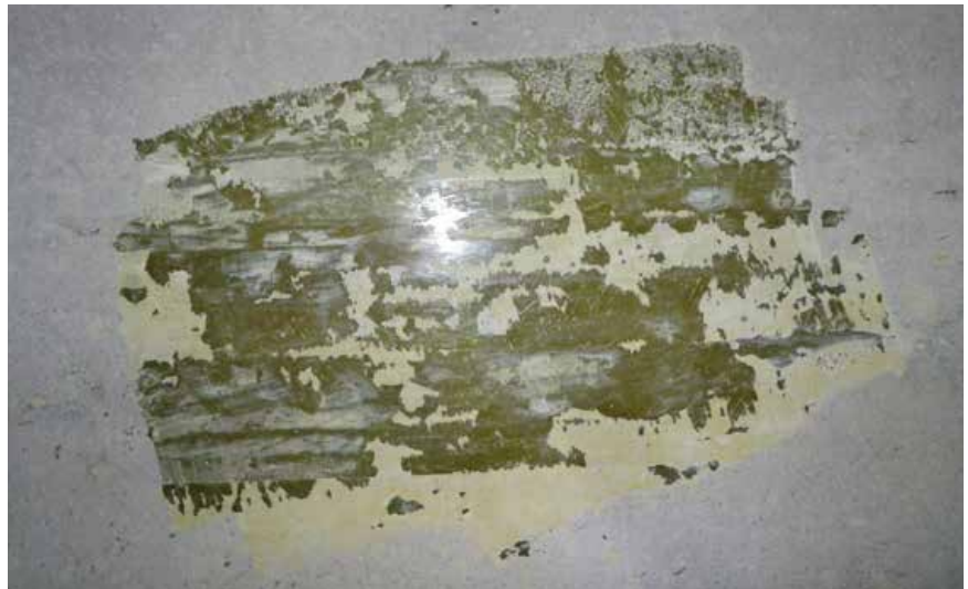
THE SHELL OF THE TANK IS COVERED IN A DRY POWDERY SUBSTANCE.
